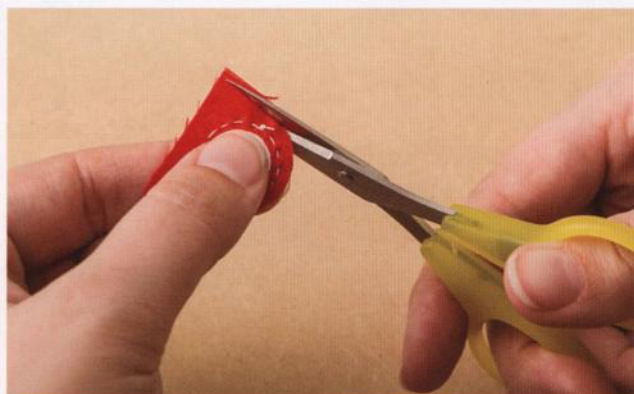
Trim the excess fabric to \frac{1}{8} " from the stitching line.
