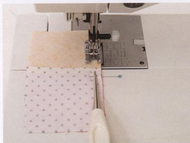
Use an awl to guide seams and keep them from flipping.
